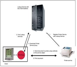
Fig. 1. Network for the Palm V PID Printer Service
