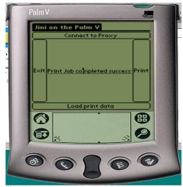
Fig. 6 Palm V PID GUI showing status of the print job
