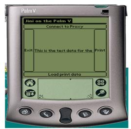
Fig. 4. A snap shot of the Palm V with its GUI for talking to the Printer Service
